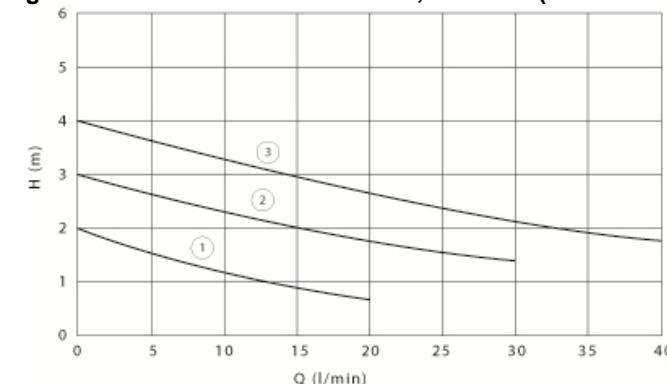
Fig. 2. Performance Curve ELS 25-6, ELS 32-6 (230V ~ 50Hz)
