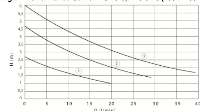
Fig. 3 Performance Curve ELS 25-8, ELS 32-8 (230V ~ 50Hz)
